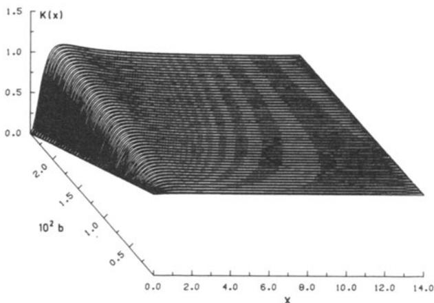
Fig. 1. Curves of the diffusion function  $K(x)$  for various values of  $x$  and laser bandwidth  $b$ .
