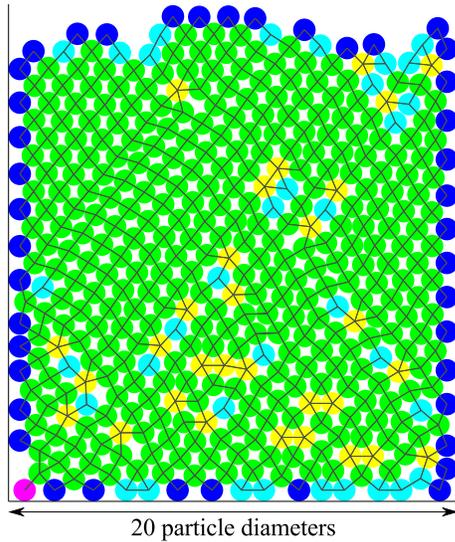
FIG. 1. A representative packing illustrating with colors the distribution of particle contacts. The particle with one contact is shown in purple, particles with two contacts in dark blue, three in cyan, four in green, and five in yellow. Vertical lines mark the limits of the channel. Bonds between particles are shown as line segments connecting their centers. Note the existence of voids (small white empty spaces).
